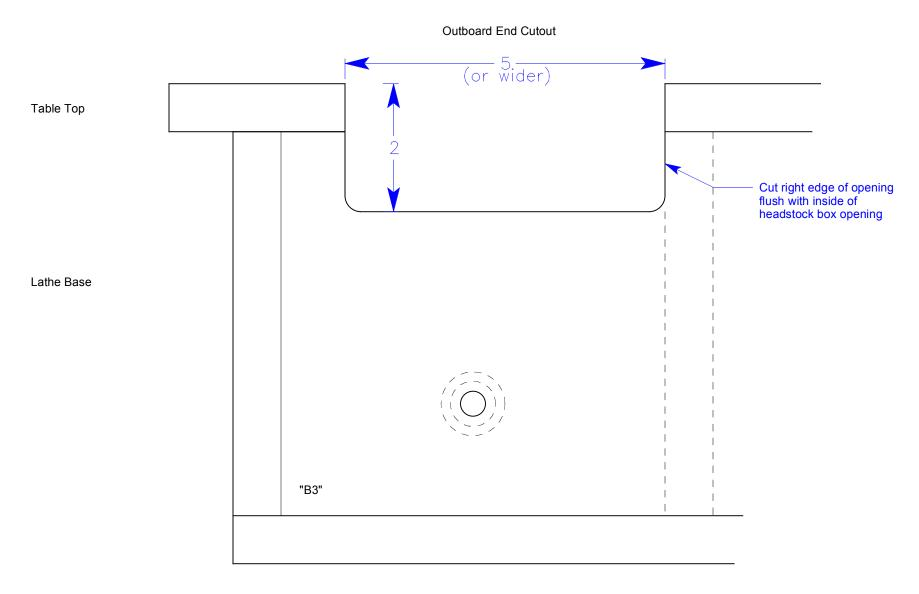
On page 2, step 2 of the Construction Instructions, drilling the holes for the pivots in the base, instead of drilling "B3" for the fixed pivot / pulley shaft, you should follow the instructions for the "B4" portion twice (last bullet point in the section) and drill the holes as described in both B3 and B4. With this modification you will be drilling for and installing two adjustable pivots, instead of the fixed pivot / pulley shaft and one adjustable pivot:
