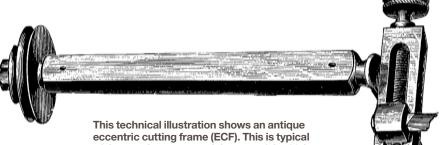
eccentric cutting frame (ECF). This is typical of the type in use around the turn of the 20th century. The knob at the top allows offsetting the cutter to increase the radius of cut. The lug on the back locks the tool holder once it has been adjusted to a given radius.
