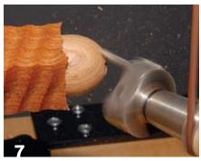
With chips flying, a modern eccentric cutting frame (ECF) uses an <sup>1</sup>/<sub>8</sub>" round carbide cutter. An example of the ECF's versatility is that it can cut a variety of hemispherical shapes merely by introducing it to the work at an angle, shown here at about 45 degrees.
