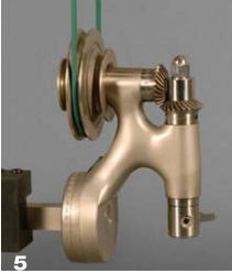
This universal cutting frame (UCF) is styled after the original design by Birch. The bevel gears on this model allow the belt to remain directed upward to the overhead drive while the cutting head can be tipped through various angles between horizontal and vertical.
