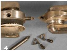
Two examples of horizontal cutting frame (HCF) cutter heads are shown *above*. Both have 60-degree tips appropriate for rose-engine work. The motorized version, *left*, uses ½" round carbide cutters. The belt-driven version, *right*, uses triangular carbide inserts borrowed from the metalworking industry.
