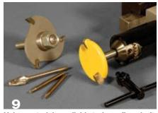
Using materials available today, a flex-shaft handpiece can be adapted to be held in the sliderest, thereby allowing use of various router bits and slotting cutters. From experience, burrs, like those pictured lower *left*, do not produce desirable patterns and should be avoided.
