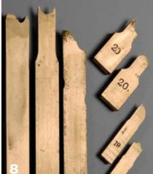
Period cutters from the heyday of OT include large-size cutting frame cutters, *top right*, stamped to indicate their 0.20" width. The small-size cutting frame cutters, *bottom right*, are often referred to as ECF cutters, as ECFs typically did not accommodate the larger sizes. The left three cutters are elaborately profiled examples of special cutters used as fixed tools in the sliderest.
