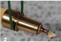
This is the typical nose of a drilling spindle with a drill in place. The belting connects to the overhead drive.
