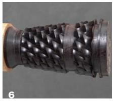
A surprising range of patterns can be created with the UCF simply by tipping it at angles. This pattern was produced using a rose-engine lathe and the UCF tilted to about 30 degrees.
