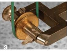
A roundnose cutter is installed in this antique vertical cutting frame (VCF).
