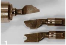
Examples of antique ornamental drills. Note the variety of profiles among these antique ornamental drills. These are all slightly offset, or cranked out, so that as they revolve, they only cut from the centerline out. The inside corner of each tip is exactly aligned with the centerline of the drilling spindle.
