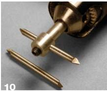
This is a simple design for a cutter to hold round carbide split-end blanks, reshaped and sharpened as desired. This one is a 1%"-diameter cutter with a 60-degree point. From readily available blanks, cutters can be made in a variety of sizes.
