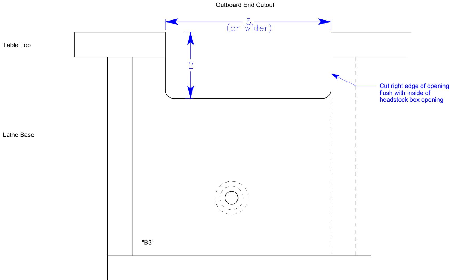
On page 2, step 2 of the Construction Instructions, drilling the holes for the pivots in the base, instead of drilling "B3" for the fixed pivot / pulley shaft, you should follow the instructions for the "B4" portion twice (last bullet point in the section) and drill the holes as described in both B3 and B4. With this modification you will be drilling for and installing two adjustable pivots, instead of the fixed pivot / pulley shaft and one adjustable pivot:
