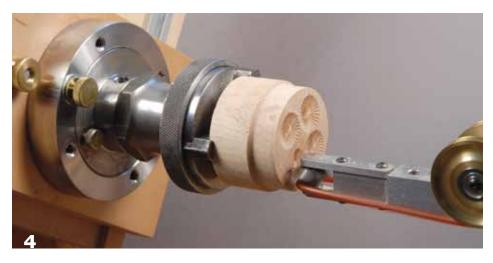
detents behind. A simpler version can be made with a disc of MDF with a 1"-8 bolt tapped through its center and mounted on a central pin allowing it to rotate. Thumbscrews around the edge can lock the disc in the desired positions. Although 96 divisions were typical on a Victorian chuck, you can get by with far fewer. Twenty-four is a versatile choice (*Photo 3*).
