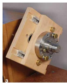
This shopmade eccentric chuck looks ungainly to most woodturners but works fine turning at 2 RPM.
