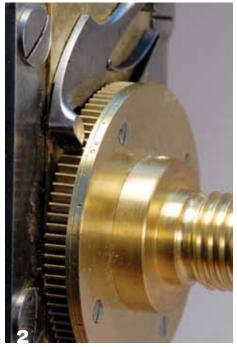
Pawl and detent style of indexing on the eccentric chuck. This one has 96 divisions, typical of most antique eccentric chucks.
