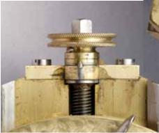
(Detail above) The eccentricity scale is engraved on the back at the bottom of the chuck. Two holes allow a tapered pin to be inserted, locking the eccentric chuck in its centered position.
