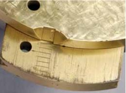
(Detail below) The adjusting knob at the top of the chuck has a small scale for fine adjustments.
