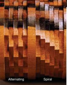
typically connected to a barrel of rosettes by a pawl. Releasing the pawl, rotating the rosette barrel to a new position, and reengaging the pawl in a detent phased the rosette. After each cut, the pawl could be released, repositioned to a new notch, and the next cut made. This quickand-easy adjustment was the key to making complex patterns in an accurate but easily repeatable fashion.
