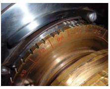
A typical notch plate on an antique roseengine lathe shows the predominant multiples of 12, and the small number of notches actually required for each group.
