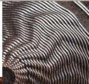
Above: To produce the moiré pattern, the notch plates or phasing holes are moved forward a few, then back a few. This moiré example is turned with a fixed cutter on African blackwood end grain.
