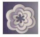
Typical angular misalignment error, exaggerated for purposes of this article, shows effects of not flattening the workpiece on the lathe.
